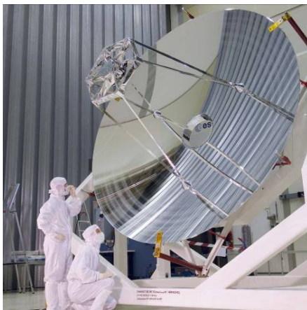
Mirror segments during preassembly and the finished mirror during the visual inspection.
