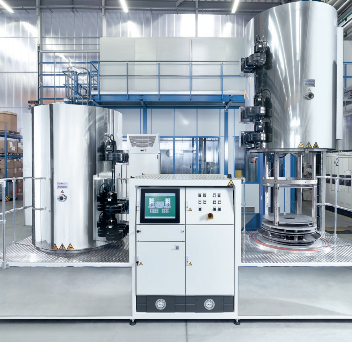
PlaTeG.Nitride 700 as tandem plant type with two separate chambers.
